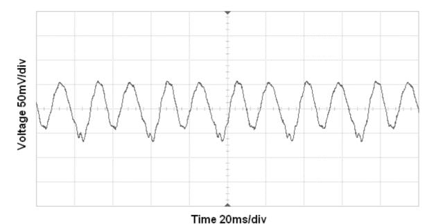
Figure 3: AC output voltage of the PFCB-W14 piezo element when loaded by  $1k\Omega$  resistor
