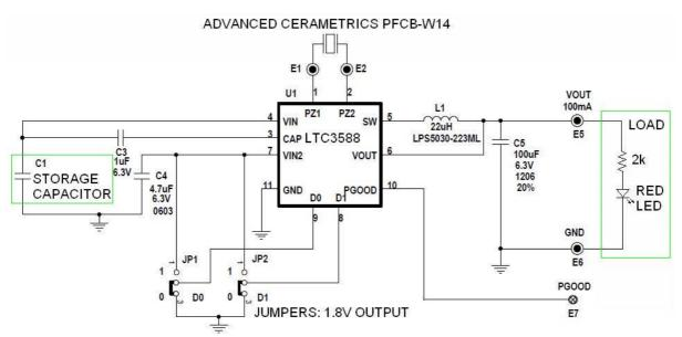
Figure 5: Schematic of the actual measuring circuit using evaluation kit DC1459B-A
