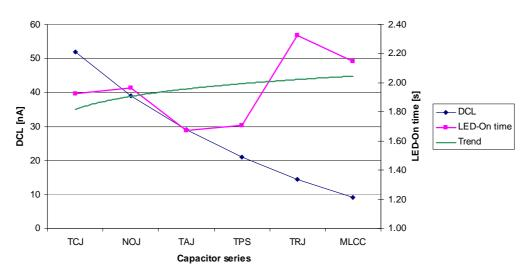
Figure 9: Storage capacitor DCL effect on LED-On time
