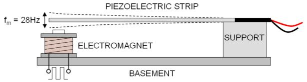
Figure 1: Experimental piezoelectric generator using PFCB-W14 element
