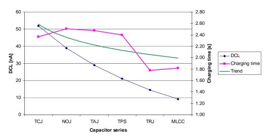
Figure 8: Storage capacitor DCL effect on charging time
