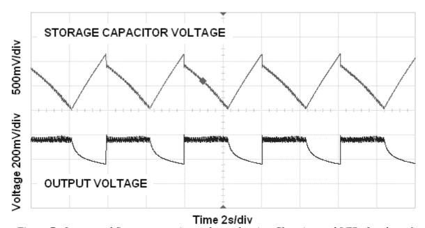
Figure 7: Output and Storage capacitor voltage showing Charging and LED-On phase for Professional Tantalum capacitor TRJB226M016R
