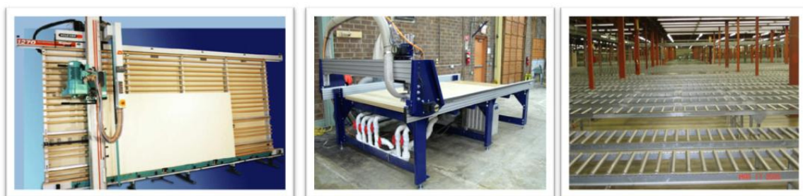
Figure 7 - From Left to Right: Linear Panel Saw, CNC Saw, Gravity Conveyor
