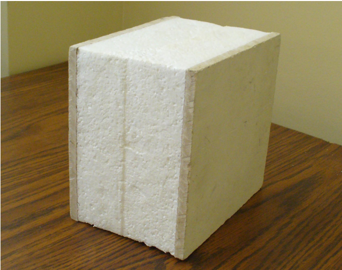
Figure 1 – Structural Insulated Panel with Cement Fiber Facing
