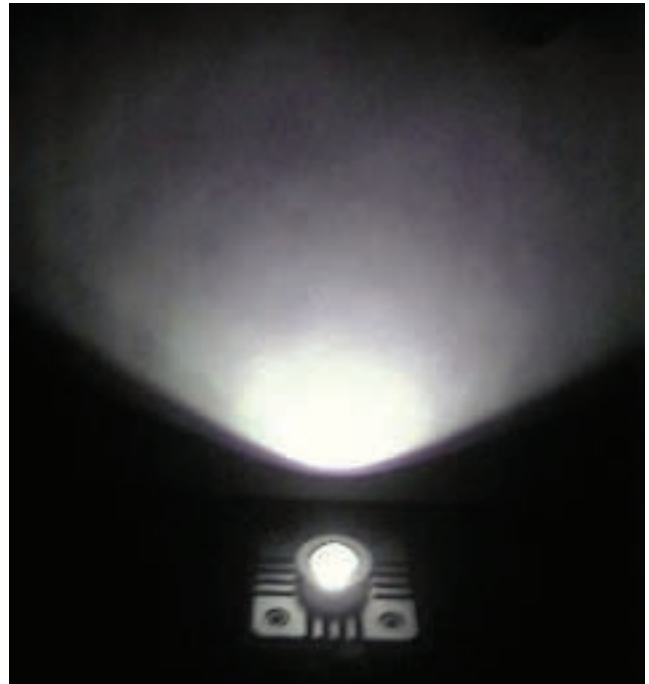
Fig. 1 A white LED using an NUV-LED and red/green/blue phosphors
