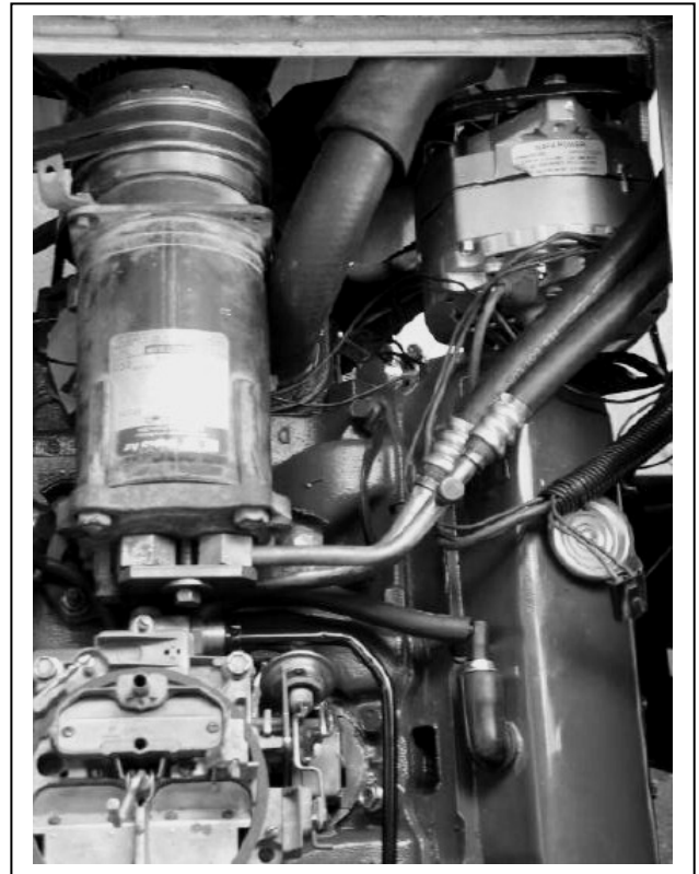
Fig. 7. Note Caddy A/C compressor location on top of the intake manifold.
