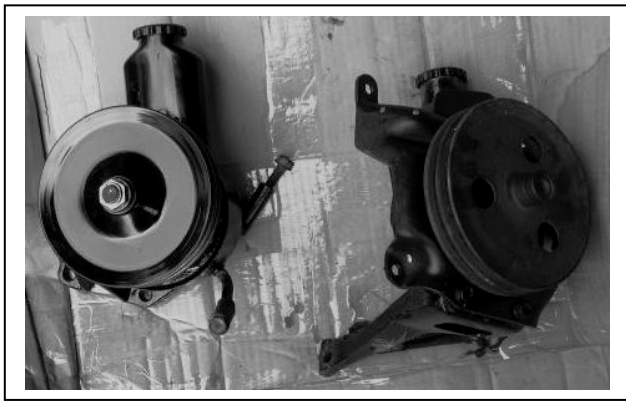
Fig. 8. Caddy PS pump on the left and GMC original on the right.
