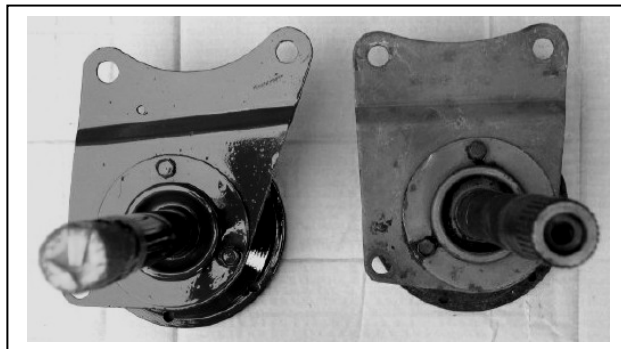
Fig 2. Caddy on the left and GMC original on the right. Note relative shape of both brackets.
