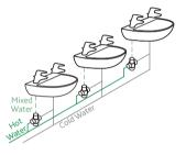
The Art 5213 thermostatic mixing valves MUST be installed in an accessible position to ensure that maintenance, commissioning and testing of the Art 5213. Thermostatic Mixing Valves can be undertaken easily.
