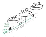
2 Consideration must be made for the possibility of multiple/simultaneous demands being made on the supply system whilst the Art 5213 valves (15 mm & 22 mm) are in use, all practical precautions must be made to ensure that the valve is not affected. Failure to make provision within the pipe sizing etc. will affect the performance of the valve.
