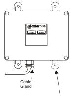
Secure using 5mm (3/16") bolts(not supplied) through the 4 mounting feet
