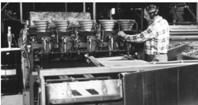
Fig. 15. Shop fabricating with fibrous glass duct liner
