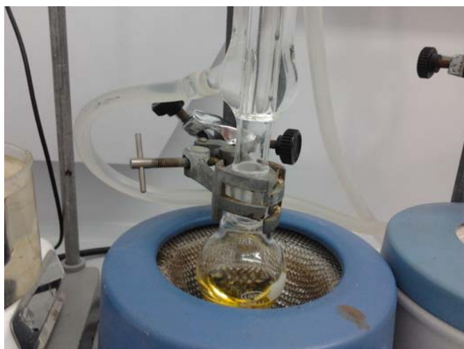
Figure SM 2.1.7.2. Reaction apparatus for the alkylation reaction
