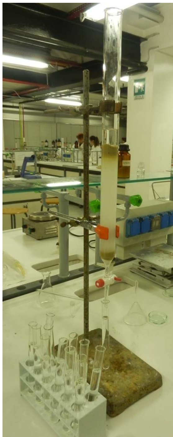
Figure SM 2.1.11.3 Column chromatography
