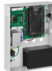
Advanced Scalable Networked Access Controller
