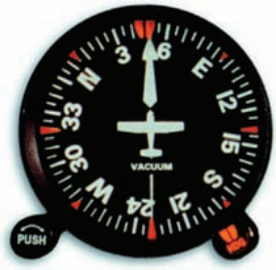
Once a vertically-mounted rotor starts to spin, it tends to stay in that alignment. The heading indicator becomes an artificial compass and gives the pilot directional information.
