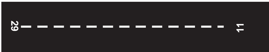
A typical VFR runway where the numbers "29" and "11" are based on magnetic headings of 290° and 110°
