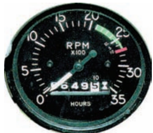
The tachometer, displaying engine speed in revolutions per minute
