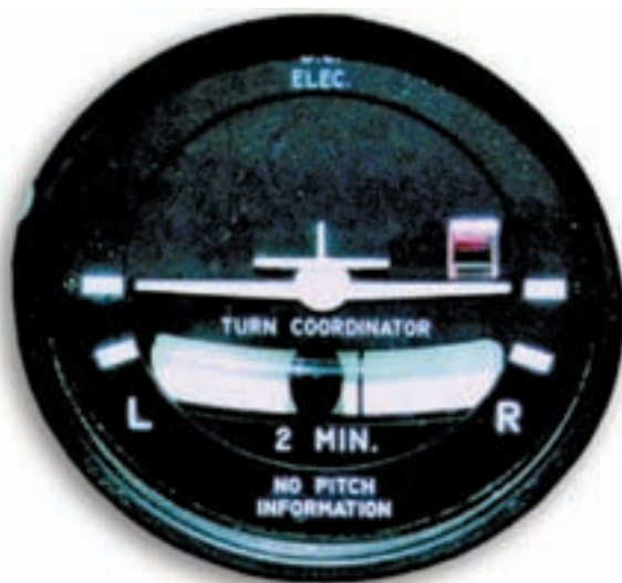
The turn coordinator uses the gyro principle for banking information.
