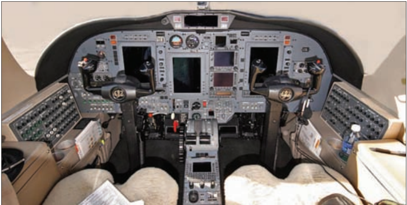
The glass cockpit of a Cessna CJ2 Citation – Image by Alex McMahon
