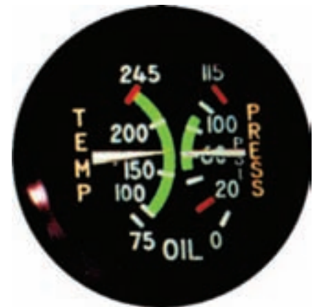
The temperature and oil pressure gauges in the cockpit
