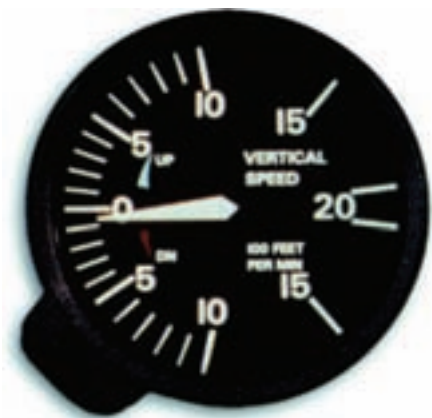
The vertical velocity indicator displays a rate of change in altitude
