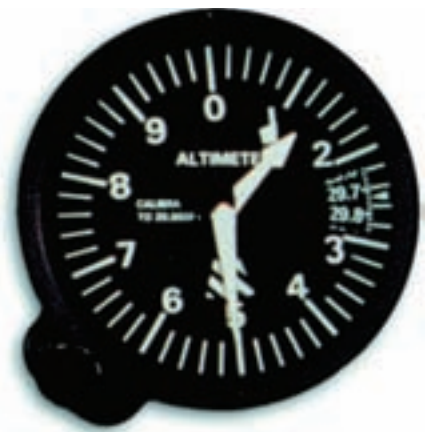
The altimeter measures pressure and displays this as height above sea level
