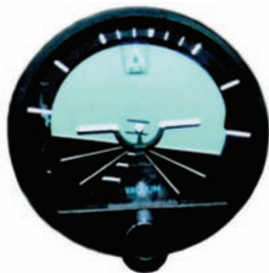
A toy gyroscope shows how it can maintain its position while spinning. When the rotor is spinning perpendicular to the surface, it is parallel to the horizon. The attitude indicator is based on this principle. It gives the pilot an “artificial horizon.”
