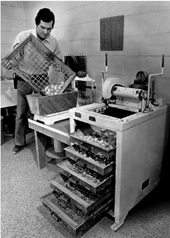
Fig. 5-5. Making a sieve analysis test of coarse aggregate in a laboratory. (30175-A)
