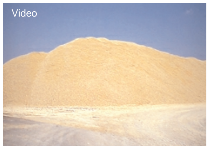
Fig. 5-24. Stockpile of aggregate at a ready mix plant. (69552)
