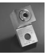
Underwriter's Laboratories Standard 486B designates connectors for use with either aluminum or copper conductors with mark AL7CU or AL9CU stamped or printed on the body of the connector. The aluminum-bodied connector to be used with aluminum conductors generally has an electrically conductive coating such as tin. Never wire-brush the connector itself.
