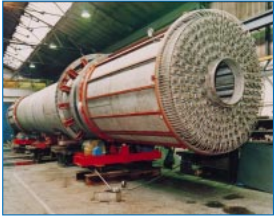
Figure 9. Fixed tube rotary dryer Photo courtesy of Mitchell Dryers Limited, Carlisle, England
