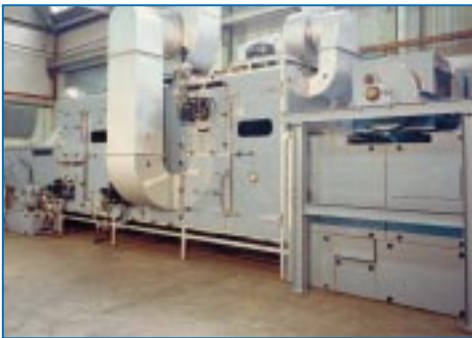
Figure 11. Continuous conveyer band dryer arrangement for direct gas firing Photo courtesy of Mitchell Dryers Limited, Carlisle, England
