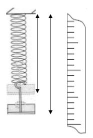
Four readings must be taken for this: the start and end point of the unloaded spring's length and the start and end point of the loaded spring's length.
