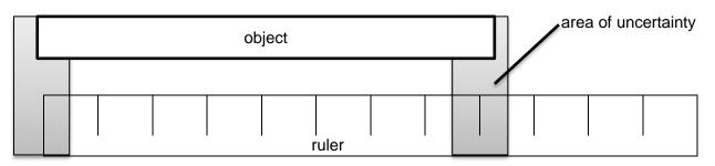
For most rulers, this will mean that the uncertainty in a measurement of length will be ±1 mm.
