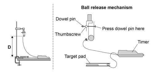
Once the ball bearing is released, the stopclock starts measuring the time. When the ball bearing hits the pad, it triggers the micro switch and stops the stopclock.
