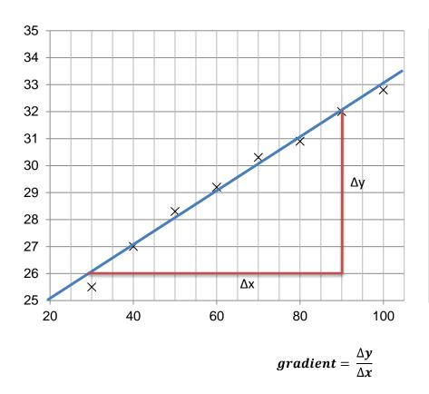
The line of best fit here has an equal number of points on both sides. It is not too wide so points can be seen under it.
