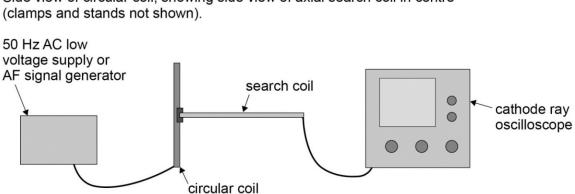
Side view of circular coil, showing side view of axial search coil in centre
