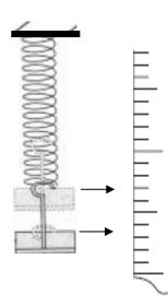
Two readings must be taken for this: the end point of the unloaded spring's length and the end point of the loaded spring's length. The start point is assumed to have zero uncertainty, as it is fixed.
