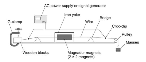
If signal generators are available, the vibration generators can be replaced by wire and magnadur magnets.
