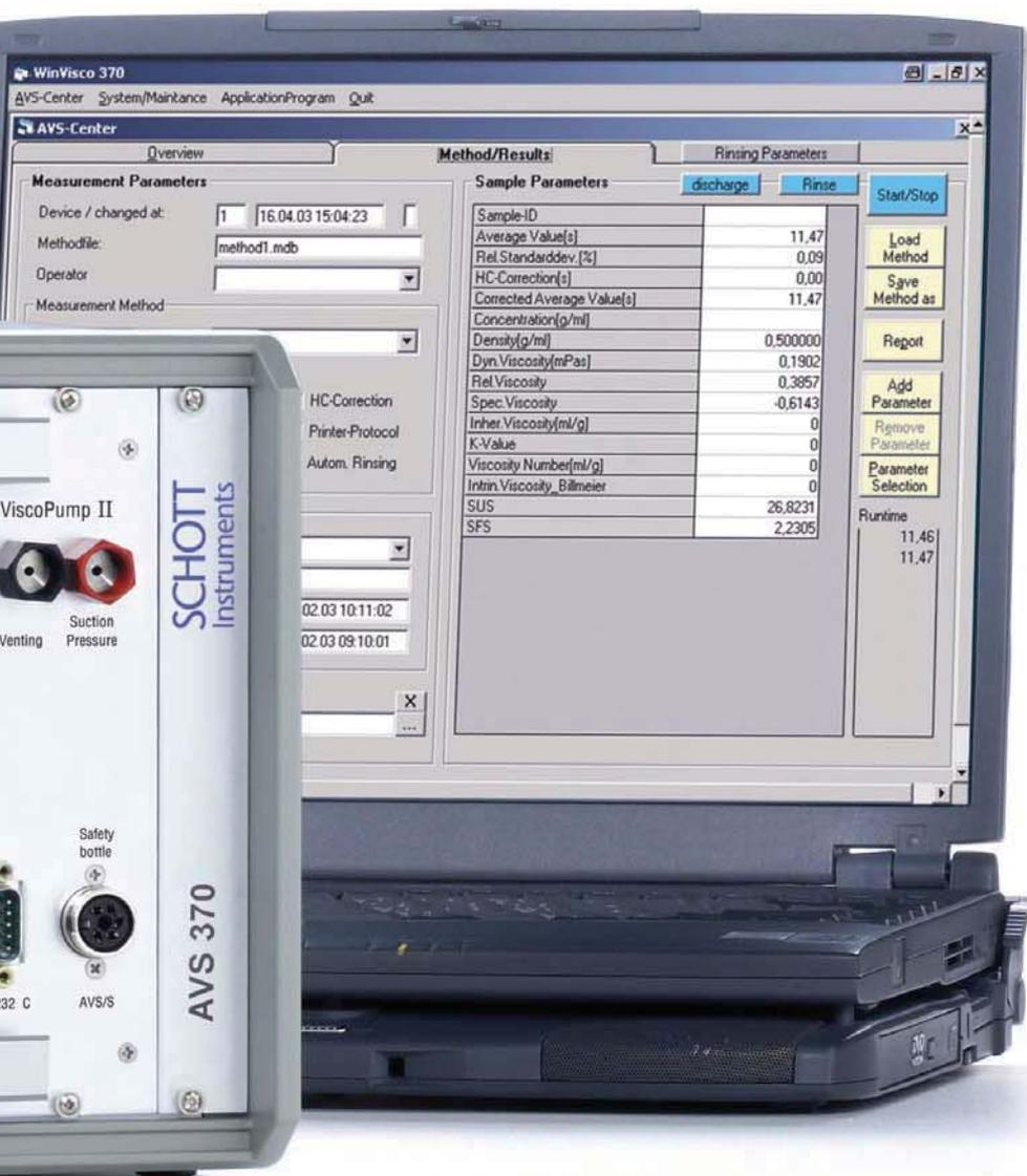
The ViscoSystem® AVS 370 from SCHOTT Instruments. Up to 4 ViscoPump II modules can be integrated in the compact 19" housing. With a PC and the WinVisco 370 software, all kinds of different samples can be measured, evaluated and documented in parallel, independently of each other.
