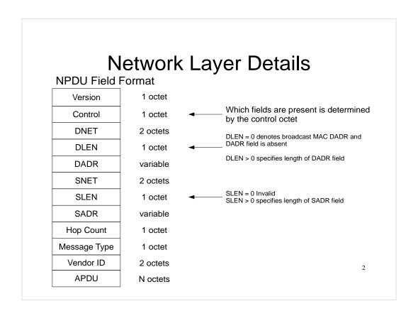
Figure 6-1. NPDU field format. Which fields are present is determined by the bits in the control octet.
