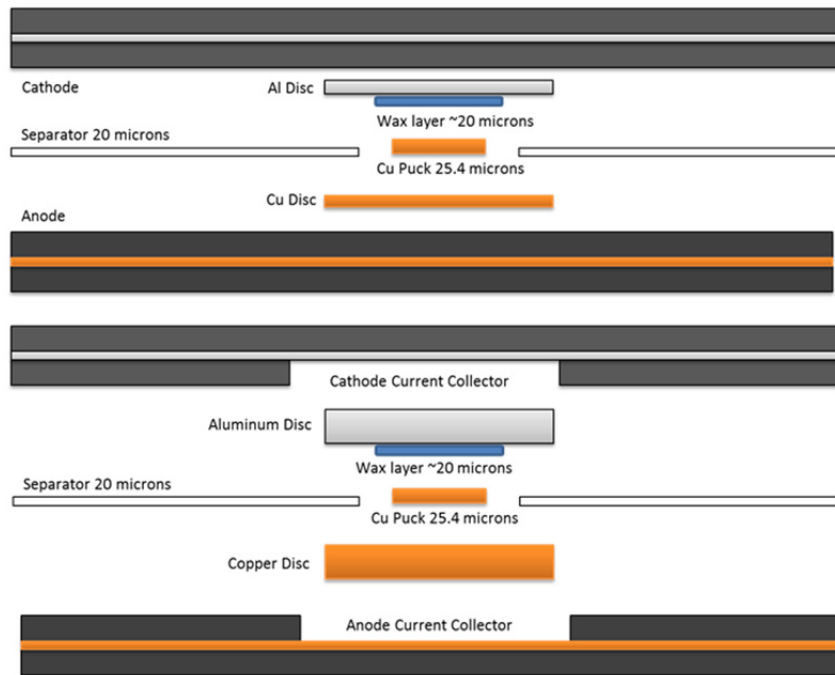
Figure IV - 53: Cathode-to-anode ISC (top) and collector-to-collector ISC (bottom) (not to scale)
