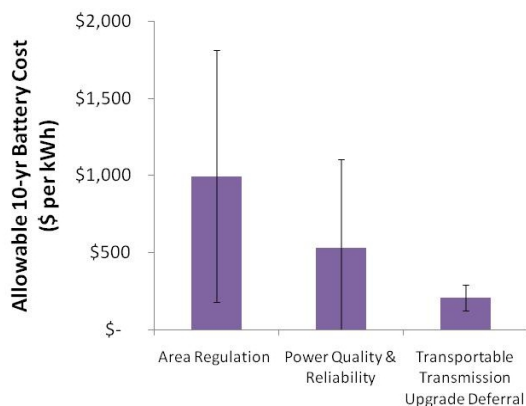
Figure IV - 10: Preliminary analysis results show multiple applications that could profitably employ second-use batteries
