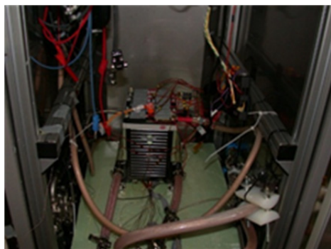
Figure IV - 84: Cell module validation test set up for LTI ROM validation against test data for US06 drive-cycle
