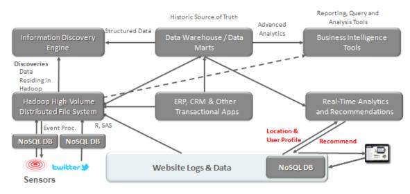
Figure 5: Integration of Hadoop Infrastructure and Data Warehouse
