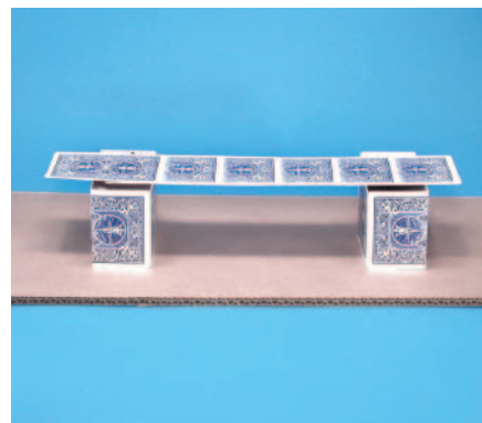
Image 2: Roadway placed across piers for test
