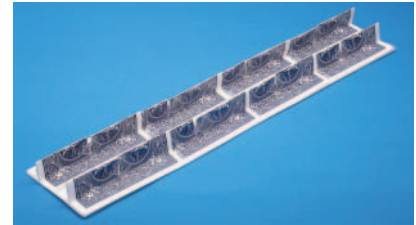
Image 1: Two long beams taped to underside of roadway
