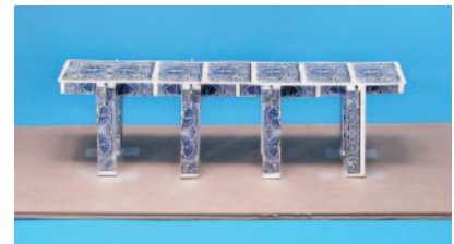
Image 4: Completed bridge with beams, crossbeams, and eight piers
