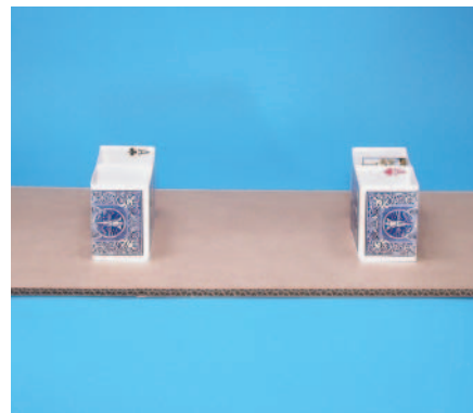
Image 1: Rectangular piers placed on cardboard base
