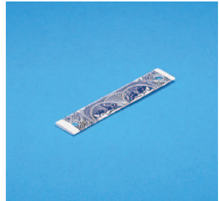
Image 3: Completed truss beam with both ends hole-punched
