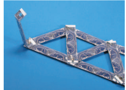
Image 2: Lateral support piece connected to truss
