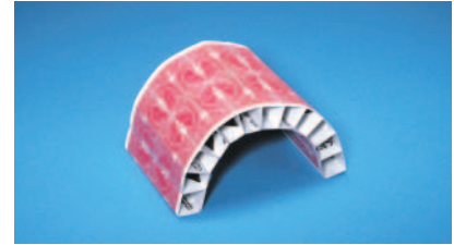
Image 2: Trapezoidal pieces stacked until they form an arch
