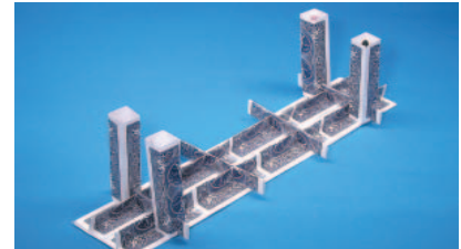
Image 2: Four crossbeams slid into slits on beams
