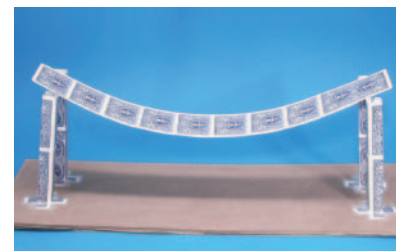
Image 3: Piers taped to base and roadway taped to piers for testing
