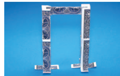
Image 1: Rectangular pier and crossbeam structure
