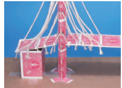
Image 3: Piers moved to outer ends of bridge and secured with tape after cables are tied
