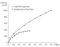
**Fig 2.** Pressure-flow properties for the high flow agarose base matrix used for Capto adhere compared to Sepharose™ 6 Fast Flow. Running conditions: BPG™ 300 (30 cm i.d.) open bed at settled bed height of 20 cm, with water at 20°C.
