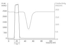
Fig 3. Buffer exchange on HiPrep 26/10 Desalting.
