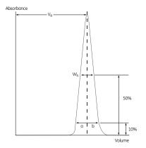
Fig 11. A typical test chromatogram showing the parameters used for HETP and  $\rm A_s$  calculations.
