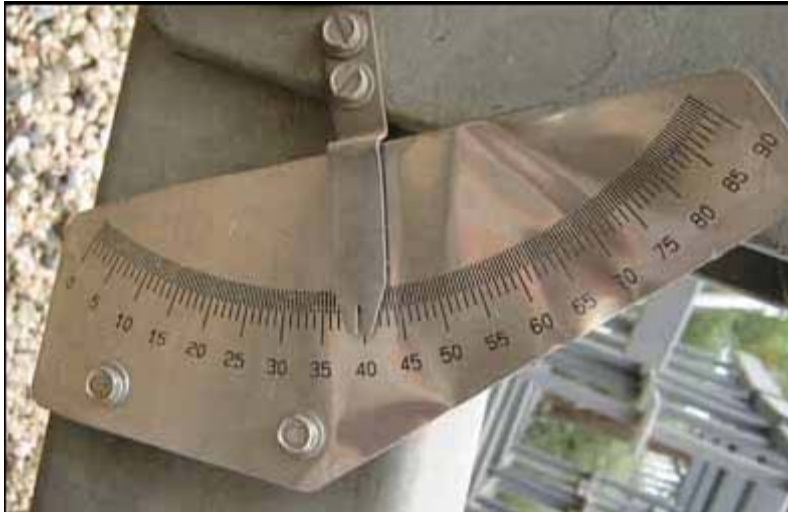
Figure 8 Angle Finder using Common Protractor
