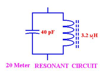
Suppose you're building a transistor amplifier stage that has an LC resonant tank circuit. Your trimmer capacitor has a range of 5 to 60 picofarads. You need an inductor that resonates with that capacitor. Let's say the band is 20 meters, 14.1 MHz. We'll design the inductor to resonate with say, 40 pF. That way, you can tweak the frequency if necessary.
