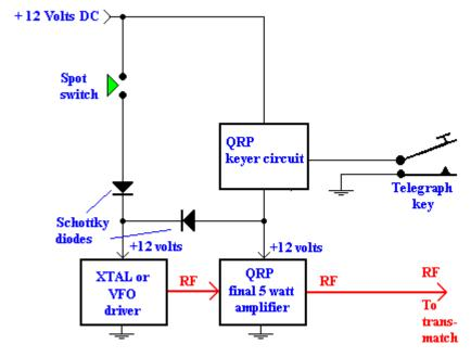
The "spot" momentary contact button turns on the oscillator buffer and with stages power through a Schottky power diode capable of handling 100 milliamperes or more. Then, when the telegraph key activates the final amplifier, the oscillator gets its power from a second Schottky diode connected to the P-channel MOSFET keyer.
