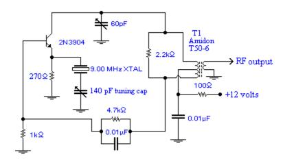
I checked out every oscillator in my receiver and transmitter and discovered that some of them didn't have the warm-up drift when turned on. The stable ones were Butler oscillators as shown on the left. Notice that the crystal and its capacitor are in parallel with the emitter resistor. I don't really know why, but this circuit is stable the moment it is turned on.
