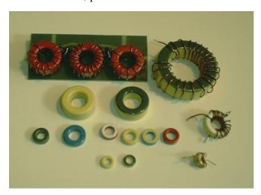
for high-Q resonant circuits and filters. Notice the powdered iron cores are color coded for their permeability. In contrast, all the ferrites are just plain black, semishiny toroid cores.
