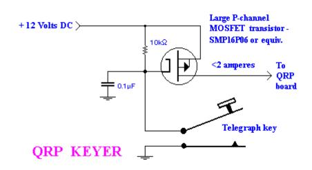
I like to key the transmitter by keying the entire power supply on and off. This circuit is not elegant, but it works. For micropower QRPs, like homebrew transmitters in Altoids boxes and sardine cans, I notice they just put the key in series with the supply. Keying the battery directly works, but for keying 5 or more watts
