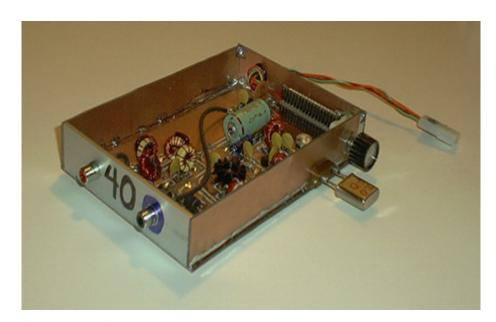
The ORP transmitter shown on the left is designed exclusively for 40 meters, (7.000 to 7.300 MHz.) The power twelve volt supply comes in through the pig-tail wire on the right. The telegraph key plugs into the bluemarked phono-plug socket on the right of the aluminum heat sink. The antenna output is the red-colored socket on the left end of the heat sink.
