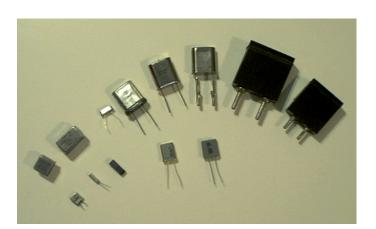
Typical crystals are shown below. Two large ancient, ham crystals are shown at the upper right. These can be good parts, provided they are still working after 50 or more years. Sometimes dead, ancient crystals in FT-243 holders can be taken
