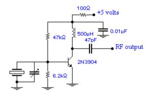
The oscillator shown on the left has the crystal connected to the base of the transistor. A variable capacitor is connected in parallel with the crystal. Again, when you first turn on the oscillator, the exact oscillator frequency may be hundreds or even thousands of Hertz off the nominal frequency. By adjusting the capacitor, the oscillation can be the exact frequency you need.
