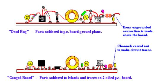
"Dead Bug" versus "Gouged Board" construction.
