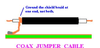
Just ground the coaxial shield at one end. The most common error when using coax jumpers on a board is to ground both ends of the shield. This introduces a "current loop" that can act something like a turn of a winding on a transformer. This current loop may pick up stray currents and the coax might do more harm than good.
