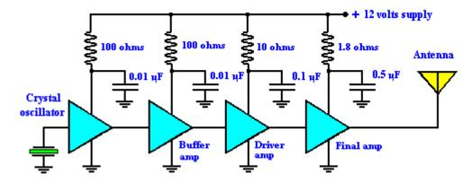
The resistor / capacitor feeding each stage slows the changes in the power supply voltage, RF cycle by cycle. That is, the R-C time constant of each network should be much longer than the variations in the power supply voltage.
