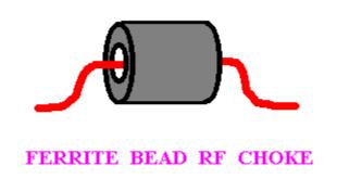
Notice the bead RF choke on the MRF-476 base. It's just a short piece of wire through a big ferrite iron bead. This eliminates low frequencies from the output and turns a "roller coaster," chaotic output waveform into a clean sinewave. This simple component looks as though it would act as a short circuit to ground. But even if you run the amplifier on a low frequency like 80 meters, the bead is vital and doesn't reduce output power. If this sounds illogical
