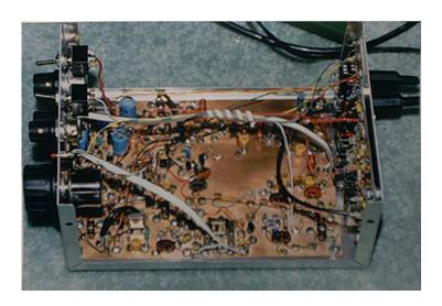
Mike Fitzgibbon, NØMF, built the homebrew QRP transceiver shown on the left using the super-glue technique. I met Mike on the air while he was using transceiver. The transceiver puts out about a watt and uses a superregenerative receiver. communicated easily across 1,400 miles so apparently it works very well.
