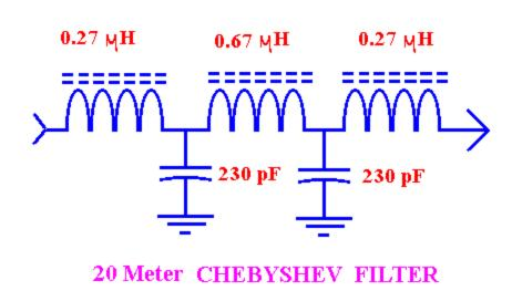
LC circuits are vital to tuned amplifier stages. But many modern amplifiers are untuned or linear and just need a filter to prevent above harmonics the transmitting frequency. The output stage of nearly every transistorized linear transmitter final has a 5-element filter to
