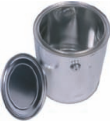
Figure 4-14. Clean, unused paint cans are often used for collecting fire debris.
