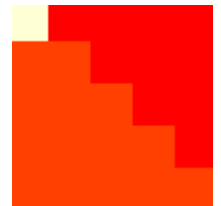
Access pattern (white) and writing pattern (yellow) for the in-place Cholesky—Banachiewicz algorithm on a 5 \times 5 matrix
