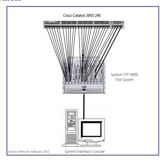
Spirent STP 9000 test ports were connected to every port on the Catalyst 3850 24S-E Switch. Three of the standards used in this testing, and which the Spirent test system incorporates, are detailed in publicly accessible RFCs. The ones most applicable to this testing include RFCs 2544 (port-pair), 2889 (full-mesh), and 3918 ("multicast) – for throughput and latency measurements of Layer 2 and Layer 3 (IPv4 and IPv6, tested separately) bidirectional traffic.
