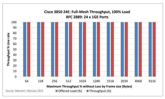
The Cisco Catalyst 3850 24S-E is able to forward full-line-rate traffic, bidirectionally, in full-mesh, round-robin fashion among all 24 fixed 1GE ports with no loss. Tests were conducted in accordance with RFC 2889.
