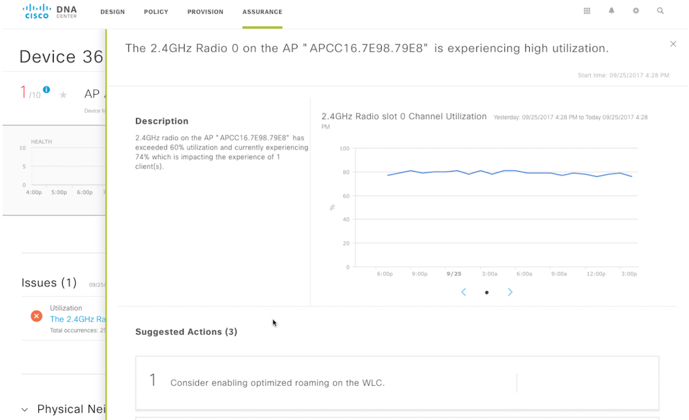
Figure 20: Root-cause identification with suggested remedies
