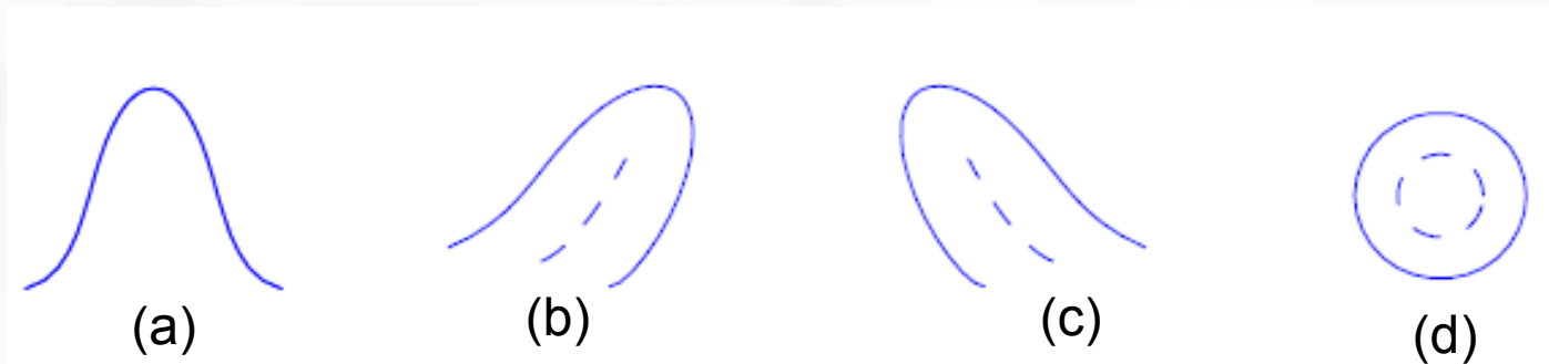
Figure: Kernels for (a) arch, (b) left-loop, (c) right-loop, and (d) whorl.
