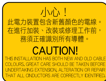
Figure A18(3) - Warning Notice
