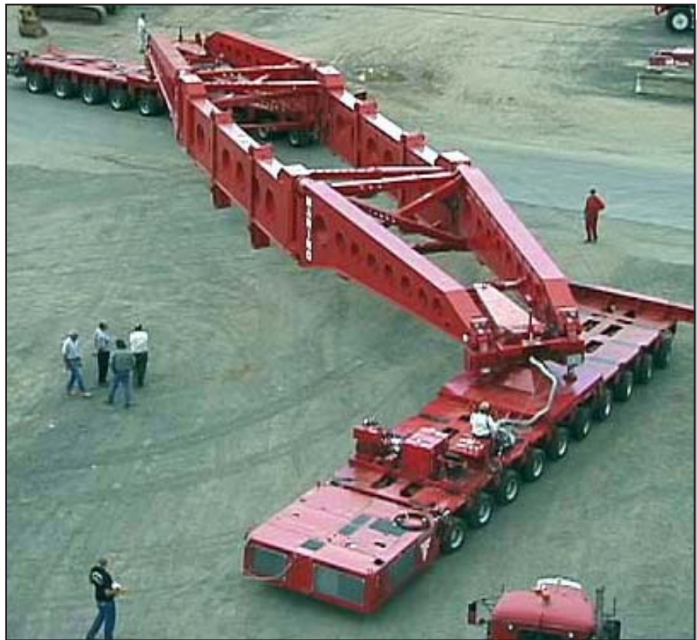
Figure 7.1-14 Goldhofer High Bridge Girder with self-propelled multi-axle trailers
