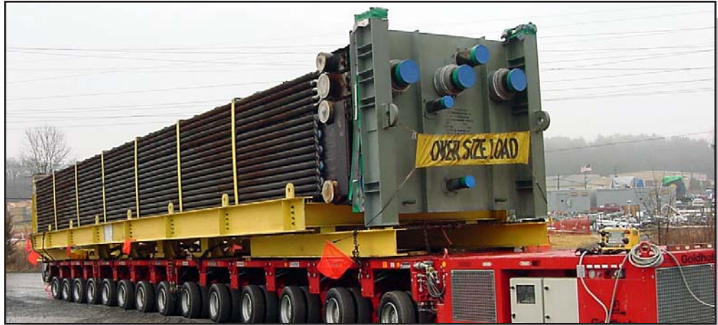
Figure 7.1-1 16-Line Hydraulic Platform Trailer Hauling a HRS Module
