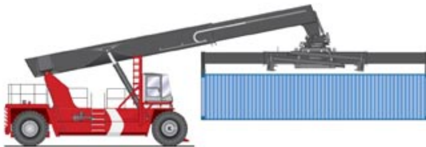
Containers can be lifted lengthwise making it possible to deliver the container into and trough workshop doors, port shed gates, etc in then low, longitudinal position.
