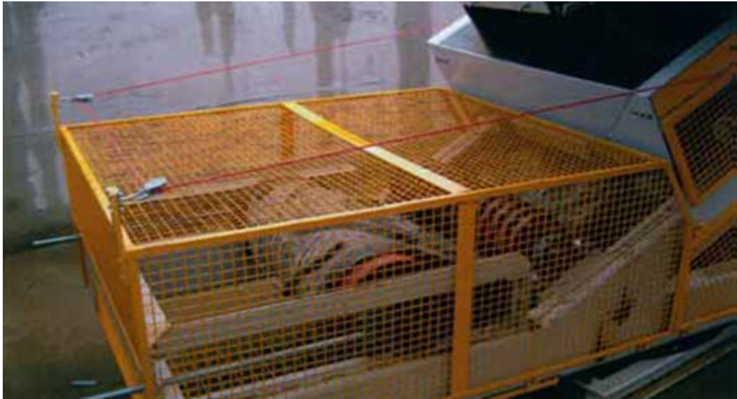
(example of fixed enclosure guard)
