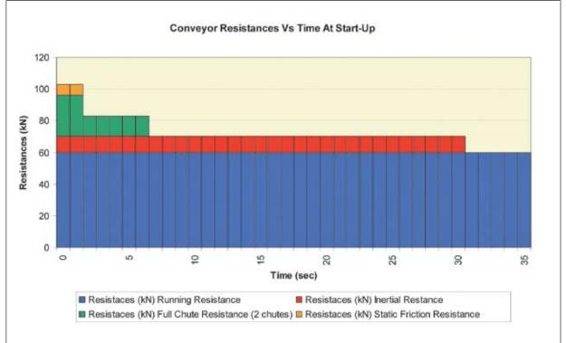
Figure 1. Example showing typical components of conveyor resistances at start-up.
