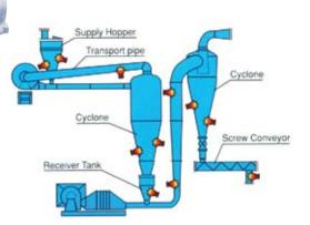
**MAGHAMMER**<sup>®</sup> is an electromagnetic hammering device. A piston moves in suspension transferring its kinetic energy to the flexible structure of the hoppers, bins, chutes, cyclones, etc. **MAGHAMMER**<sup>®</sup> prevents clogging and adhesion of powdery and granular materials in hoppers, ducts, chutes, cyclones, etc.
