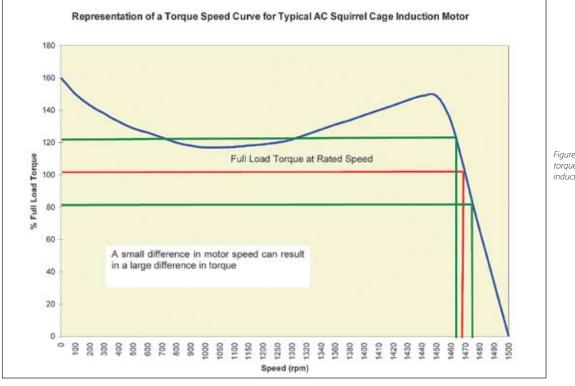
Figure 3. Representation of a typical torque speed curve for a squirrel cage induction motor.
