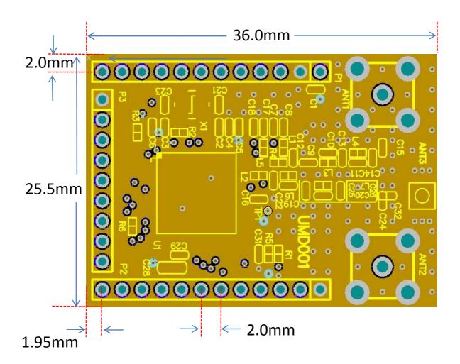
Dimensions : length 25.5 mm X width 36mm X height 3mm
