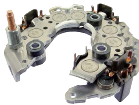
31-82054 Rectifier 117mm OD, 6mm Top Post 100 Amp, 12 Diodes
