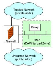
Figure 24 Firewall traversal
