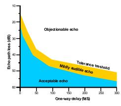
Figure 16 Talker echo tolerance as function of delay
