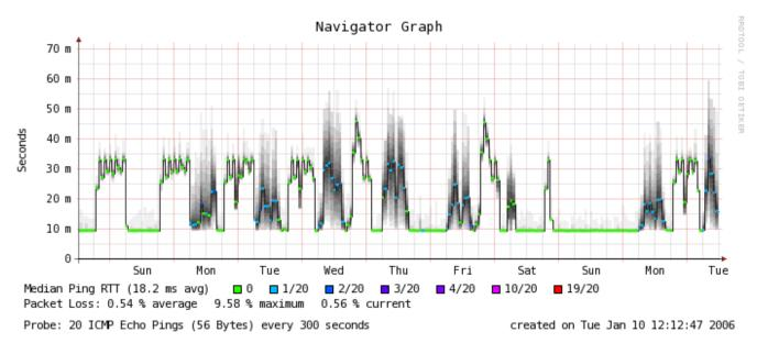
Figure 30 Delay and packet loss measurement
