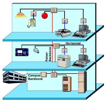
Today buildings are usually cabled using a structured cabling system (See reference 1). A structured cabling system is a standard for cable design. The main concept of structured cabling is to have a standard cabling infrastructure that can be used for the data network, the telephony network and the building management.
