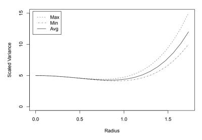
Figure 10.6 Fraction of Design Space Plot for Box-Behnken Design in Three Factors
