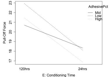
Figure 12.13 Interaction between D=Percent Adhesive and E=Conditioning Time
