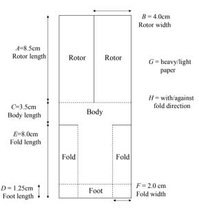
Figure 6.19 Standard Helicopter Design
