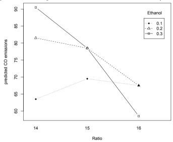
Figure 3.7 Linear by Linear Interaction Plot Ethanol and Air/Fuel Ratio
