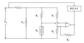
response, or measure of product performance, is the resistance value of  $R_T$  at which the relay turns on. Through circuit relations, the response is given by the rational function
