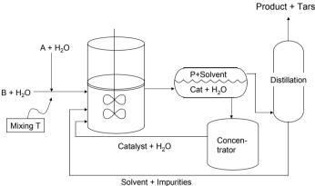
Figure 3.14 Diagram of a Chemical Process
