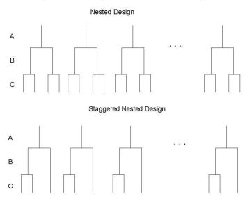
nested design increases. Figure 5.2 shows the schematic for staggered nested designs from three through six stages.
