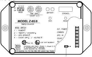
Jumper switch location for .1 - 9.9 counts (x.x) factory positioned
