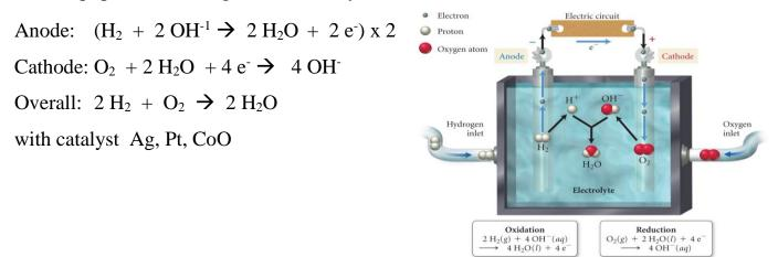
Newer fuel cells replaced the strong OH<sup>-1</sup> electrolyte with a special proton exchange membrane (PEM).
