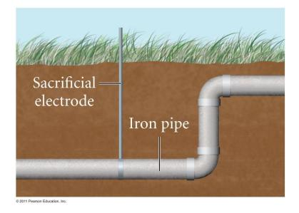
Problem: Over time the sacrificial anode corrodes and will need to be replaced.
