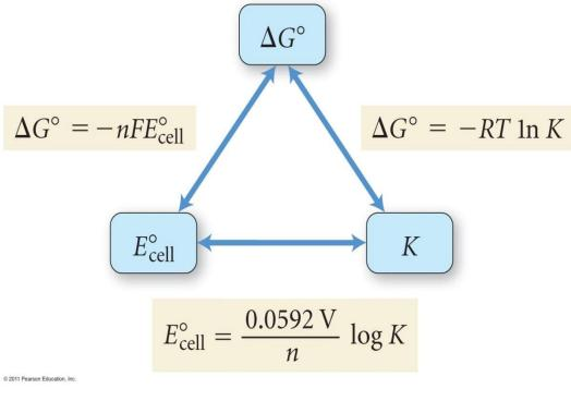
or  $E^{\circ}_{cell} = (0.0257/n) \ln K_{eq}$  at 25°C
