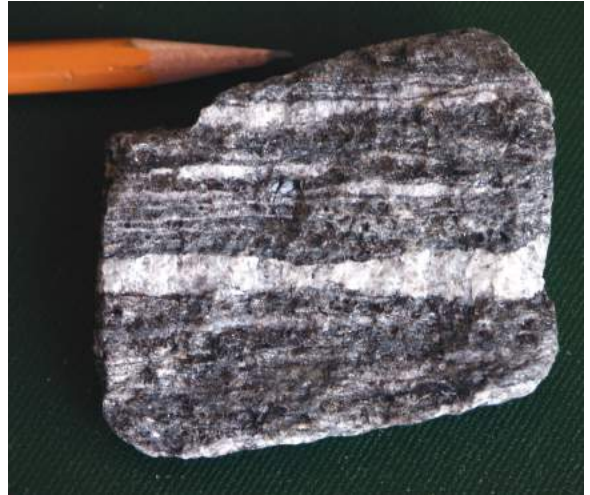
FIGURE 5-13. Gneiss is a metamorphic rock that is often composed of minerals separated into light- and dark-colored bands. The light bands are rich in feldspar and quartz. Amphibole and pyroxene are the primary minerals in the dark bands.
