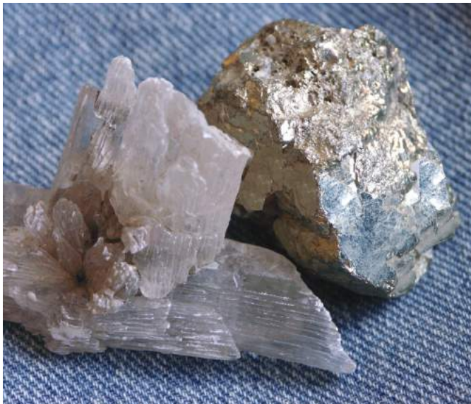
FIGURE 4-6. Selenite gypsum has a glassy luster because it is translucent. Pyrite has a nontransparent metallic luster.
