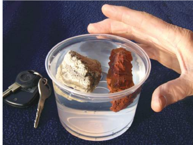
FIGURE 5-6. Pumice (right) and scoria (left) are vesicular (contain small air pockets), igneous rocks. Sometimes they have so many vesicles that these rocks will float on water.
