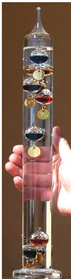
FIGURE 1-8. This instrument is a Galileo thermometer. As the water inside becomes warmer or cooler, it changes in density. So the number of glass spheres that float changes.
