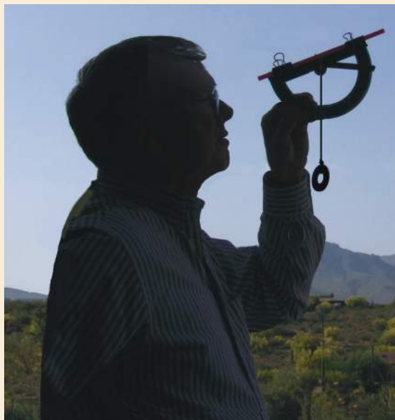
FIGURE 2-11. To make a simple celestial navigation instrument, use protractor, a drinking straw, and a weight on a string.
