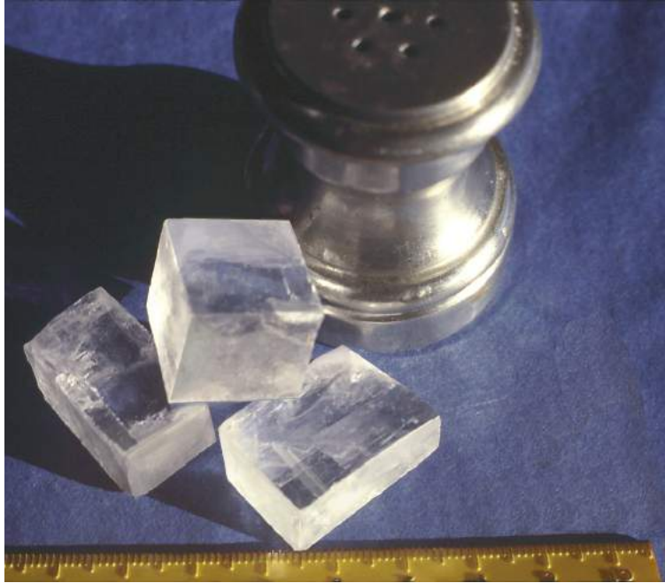
FIGURE 4-9. Halite, also known as rock salt, forms cubic crystals that also break (cleave) into rectangular solids.
