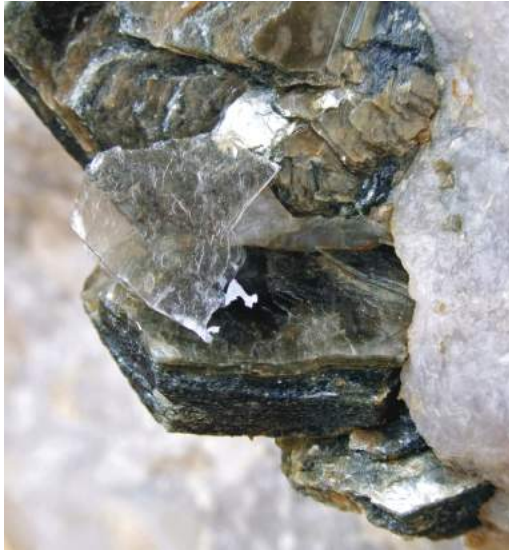
FIGURE 4-8. Muscovite, like other minerals in the mica family, has perfect cleavage in one direction. That is, all mica minerals split into very thin, flexible sheets.
