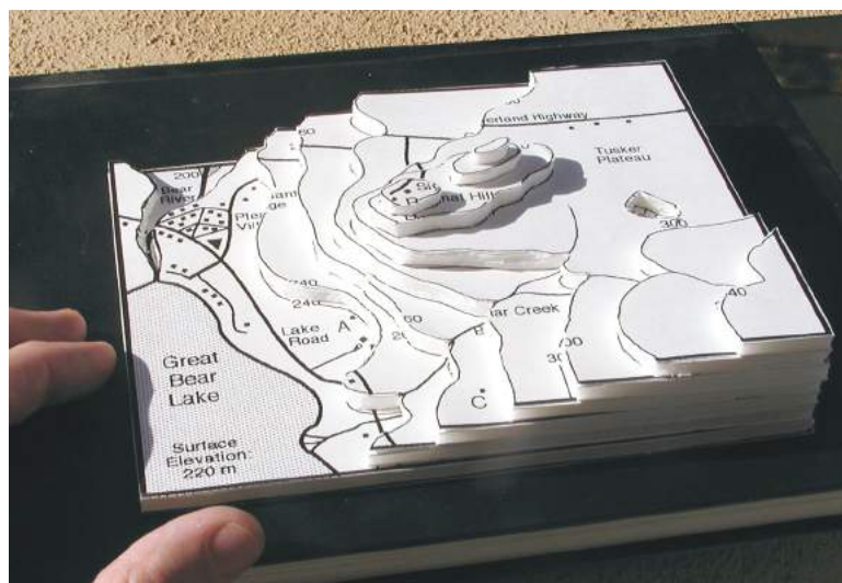
FIGURE 3-7. You can make a three-dimensional model of any topographic map or land surface using sheets of foam available at art supply stores or from supermarket food trays.
