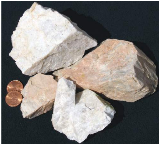
FIGURE 4-11. Plagioclase and potassium feldspar are extremely common, both gave a glassy luster and show cleavage at nearly 90°.
