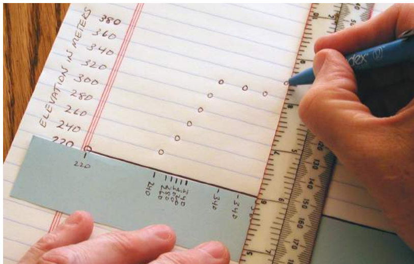
FIGURE 3-14. After labeling each mark with the elevation of the contour line it represents, the next step is to draw a dot at the correct elevation on the lined paper.
