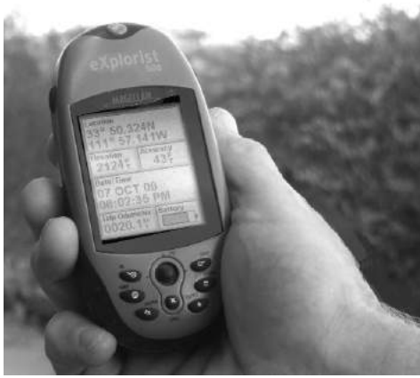
FIGURE 1-14. A global positioning system receiver processes signals from satellites to determine your precise location on Earth.
