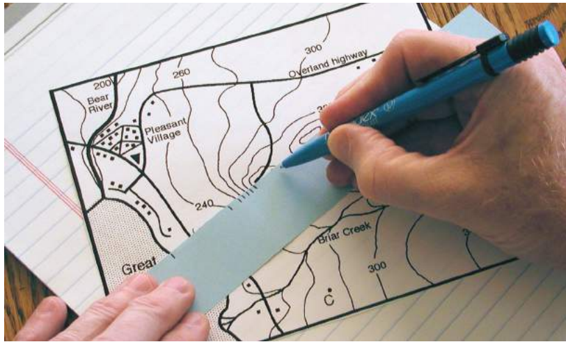
FIGURE 3-13. The first step in making a profile from a contour map is marking the blank strip where it crosses each contour line.
