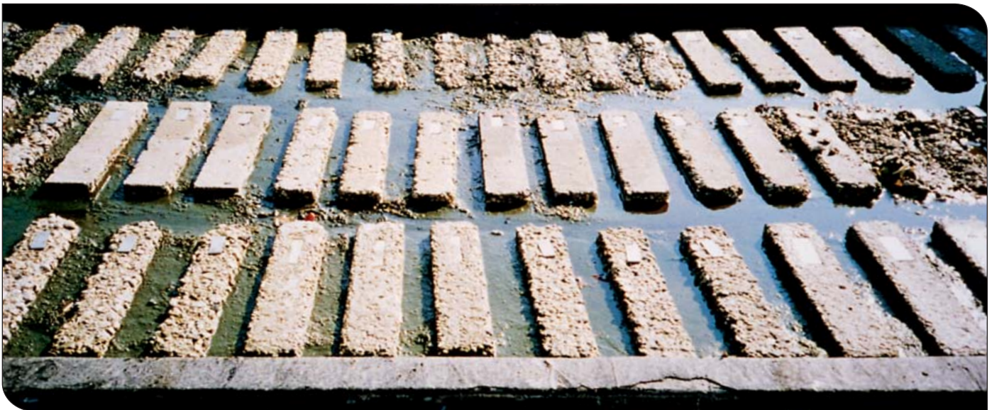
Fig. 1. Aggressive substances can compromise the durability of concrete. Shown are concrete beams exposed to high-concentration sulfate soils/solutions. (PCA/CALTRANS test plot, Sacramento, California) (Stark 2002) (IMG12296)
