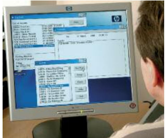
Automatic test systems facilitate testing of emergency lighting, though need to be compliant with IEC 62034
