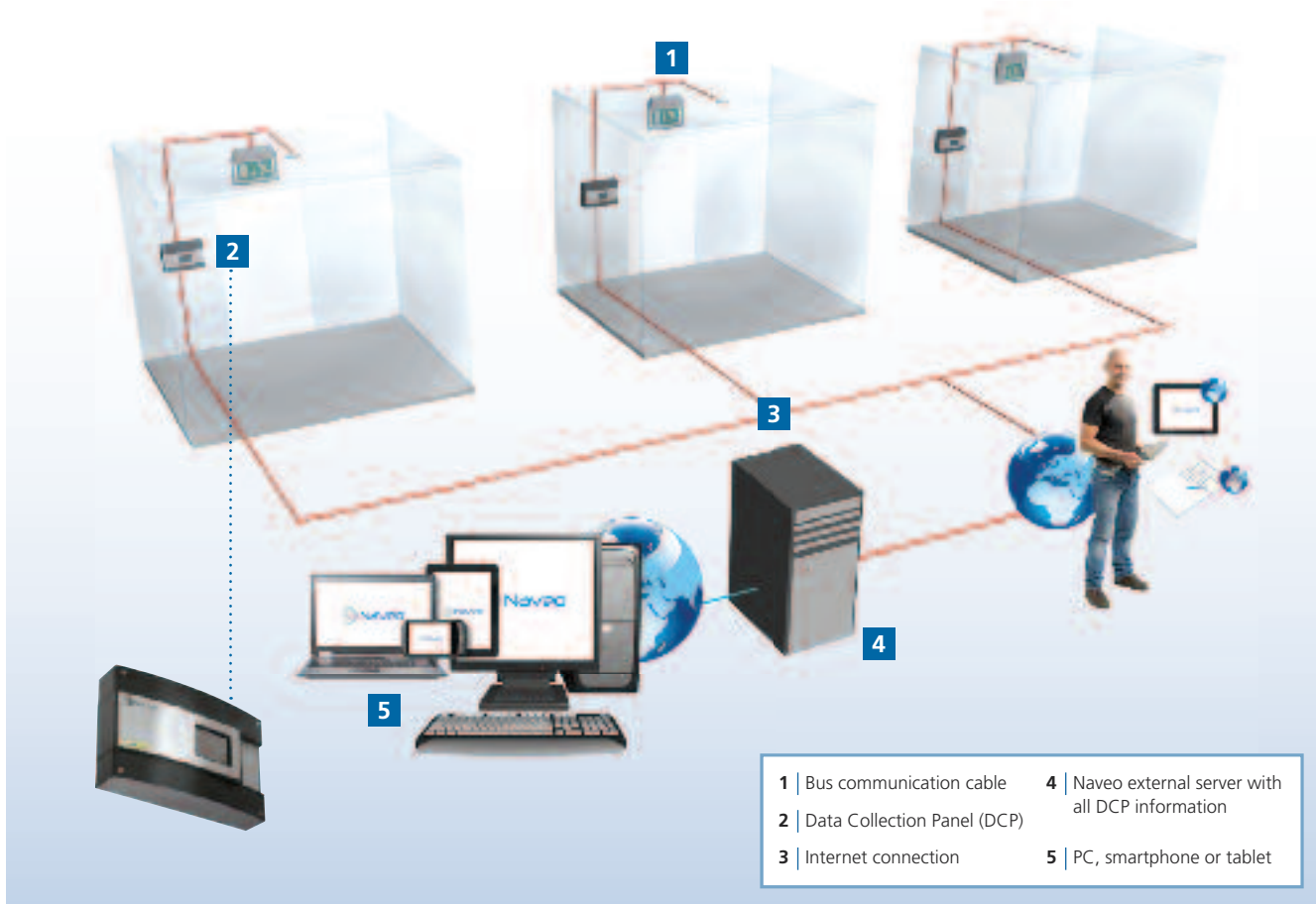
Figure 40: Emergi-Lite Naveo addressable test system with remote monitoring and management
