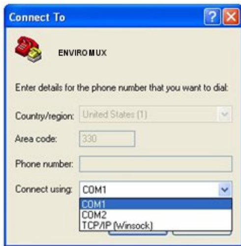
Figure 11- Configure COM port in HyperTerminal
