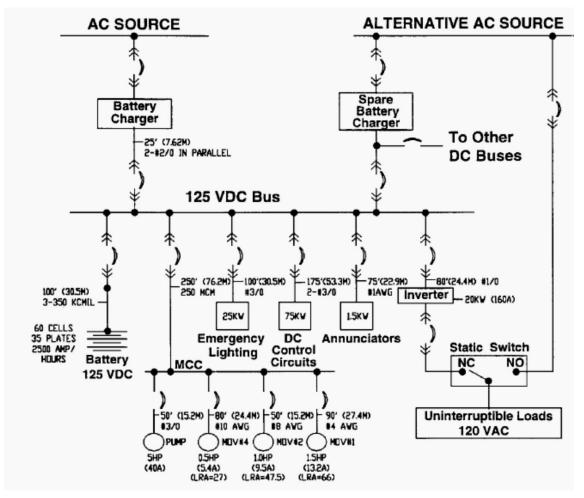
Figure 1: Sample dc one-line diagram from IEEE 399-1997
