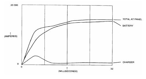
Figure E.1—Typical fault-current contributions at the dc bus with current-limited charger
