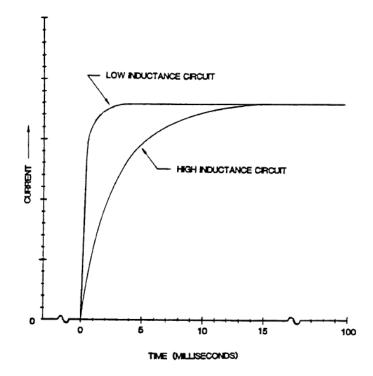
Figure 5: Early Battery response to a short circuit (C&D)
