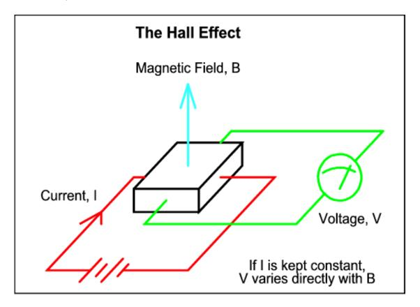
What can you do with a Hall-effect device? Build an electronic circuit which will amplify the voltage across the device and calibrate it so you can measure a voltage and translate that into a Gauss measurement. For such a unit, check out the page on building a <u>Gaussmeter</u>.
