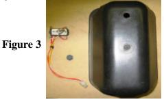
Tow/Run switch, mounting nut, and cover after disassembly
