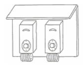
To get the desired temperature, thermostats should be located at plant height near the center of the greenhouse where they are not influenced by drafts or sidewall cooling. It is best if both the thermostat and speed control are located together and protected from direct contact with sunlight and water. One simple way to accomplish this would be to mount the controls to a piece of wood with a top on it like in the picture to the left. Wood should be painted white to shade it from the sun.
