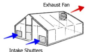
The picture to the left shows optimal fan and shutter placement in a greenhouse. The exhaust fan should be mounted near the peak so that it is exhausting the hottest air in the greenhouse. The intake shutters should be mounted on the opposite end of the greenhouse so that the cooler fresh air travels across the entire structure minimizing hot spots.
