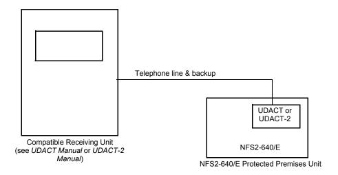
Figure 4.4 Typical Proprietary Fire Alarm Systems Wiring Connections
