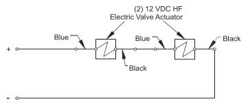
Figure 4.9 Releasing Circuits (Option 2)
