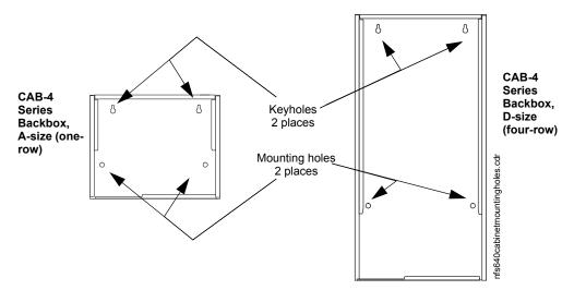
Figure 3.1 Mounting Holes of a Backbox
