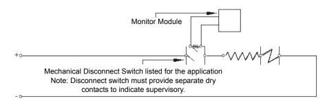
Figure 4.11 Release Circuits (Mechanical Disconnect Switch)
