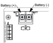
Figure 3.15 CPS-24/E: DC Power Connections
