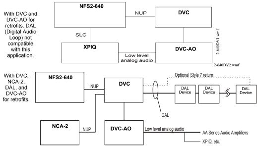
Figure 3.13 Block Diagrams of DVC Series Applications
