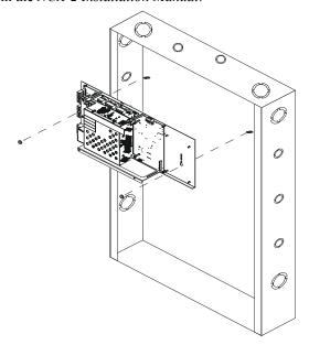
Figure 3.4 NFS2-640/E Chassis Mounting
