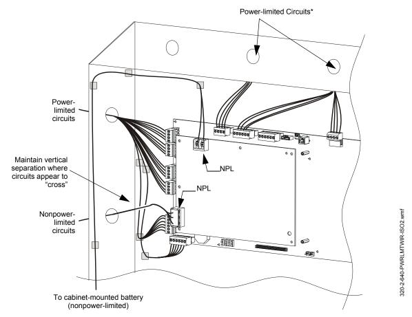
Figure 3.22 Typical Wiring for UL Power-limited Wiring Requirements (Shown with relays as connected to power-limited modules)
