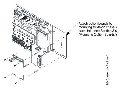
Figure 3.7 Attaching Option Boards to the Right of the CPU
