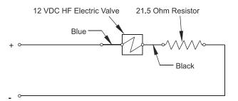
Figure 4.10 Releasing Circuits (Option 3)
