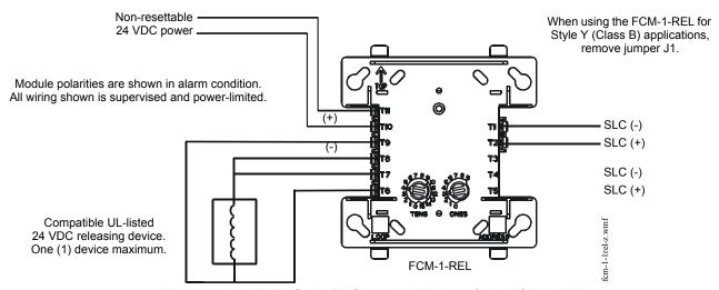
Figure 4.13 NPFA Style Z (Class A) Wiring of the FCM-1-REL
