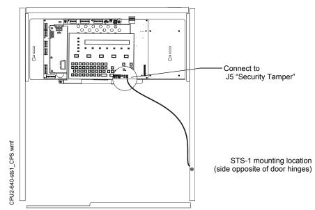
Figure 4.5 Installing the STS-1 Security Tamper Switch
