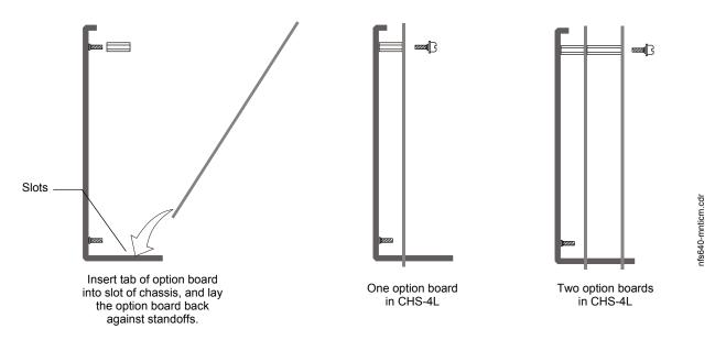
Figure 3.9 Mounting an Option Board in a Chassis (CHS-4L Shown)
