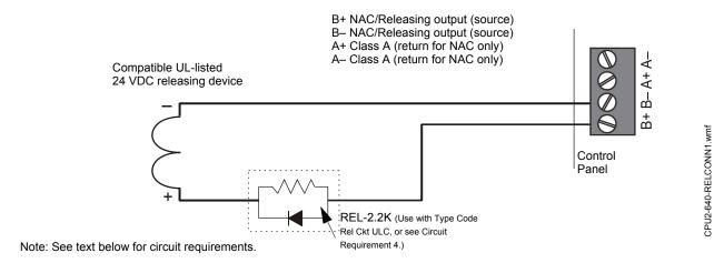
Figure 4.7 Typical Style 4 Connection of a Releasing Device to Control Panel
