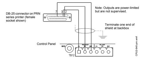
Figure 3.24 Remote Printer Connections
