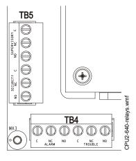
Figure 3.20 Form-C Relay Connections
