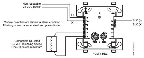
Figure 4.13 NPFA Style Y (Class B) Wiring of the FCM-1-REL
