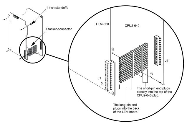
Figure 3.12 Mounting LEM-320 with the Stacker-connector
