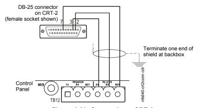
Figure 3.26 Connecting a CRT-2
