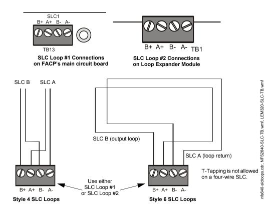
Figure 3.28 SLC Loop Connections and Wiring
