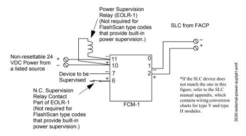
Figure 4.1 Enabling External Power Supervision Using Relays
