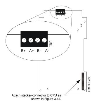
Figure 3.11 SLC Connections for LEM-320
