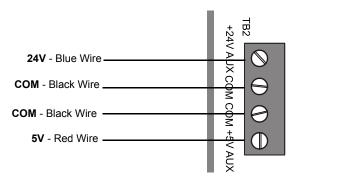
Figure 3.17 Connecting to the Accessories Output TB2 on CPS-24/E
