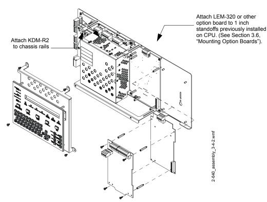
Figure 3.6 Attaching Option Boards Behind KDM-R2
