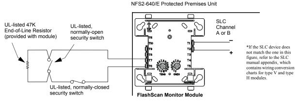
Figure 4.6 Wiring Diagram for Proprietary Security Alarm Applications
