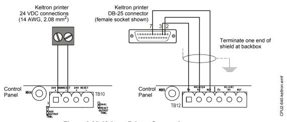
Figure 3.25 Keltron Printer Connections
