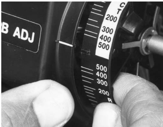
Figure 4-2. Changing Controller Action on Fisher 4195KB and KC Controllers
