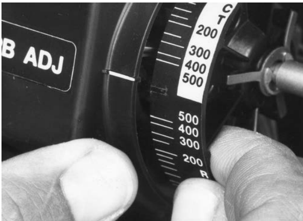
Figure 3-2. Changing Controller Action on Fisher 4195KA Controllers
