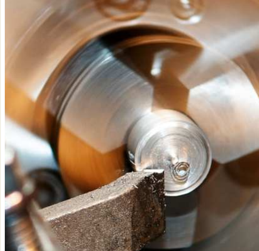
Counterbores for solderless tube connection (DIN 3854/DIN 3862)
