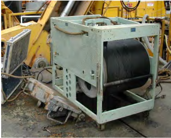
Plate 8.2 – Device for Ultrasonic Echo Sounding Tests
