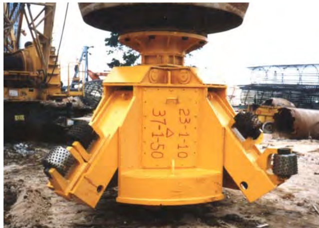
Plate 8.1 – A Mechanical Bell-out Tool
