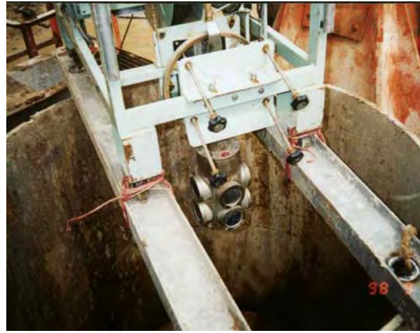
Plate 8.3 – Sensor for Ultrasonic Echo Sounding Tests
